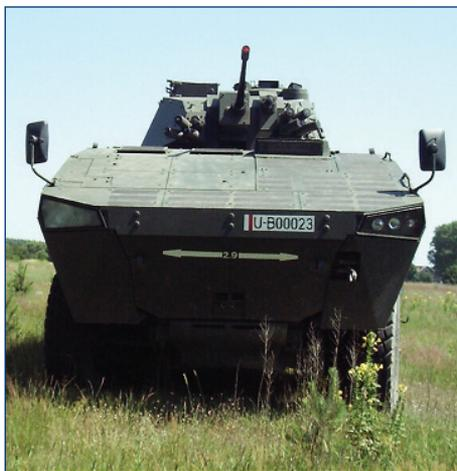
The armoured 120 mm twin mortar system is called AMOS-FIN. The industrial cooperation is executed by the Finnish Patria and the Swedish Alvis Hägglunds. The basic idea of the mortar vehicle was to develop a mobile unit of indirect fire with capability to open quick fire. The special requirement was to enable burst of fire so that all grenades fired during the firing have their
