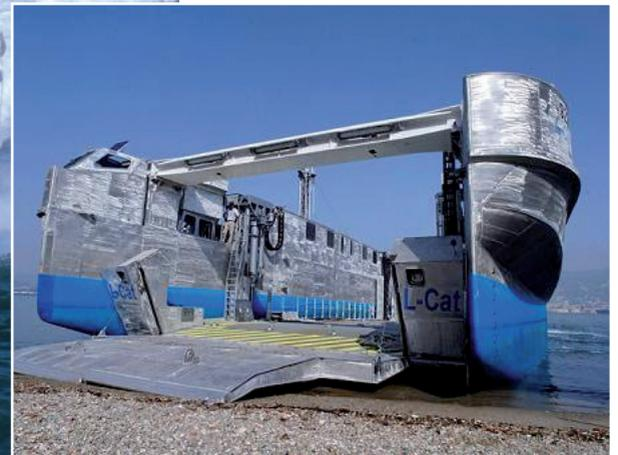
good sea keeping capabilities and a large capacity (two Leclerc tanks and four VBL or six VAB); it enables landing from a BPC situated over the horizon. This innovative concept, combining catamaran and mobile platform is so far unique in the world.
